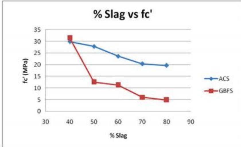
**FIGURE 3.** Compression strength results of geopolymers, prepared from various ratio air-cooled slag or granulated blast furnace slag to fly ash and alkali activator (NaOH 12M and water glass 10 M).
