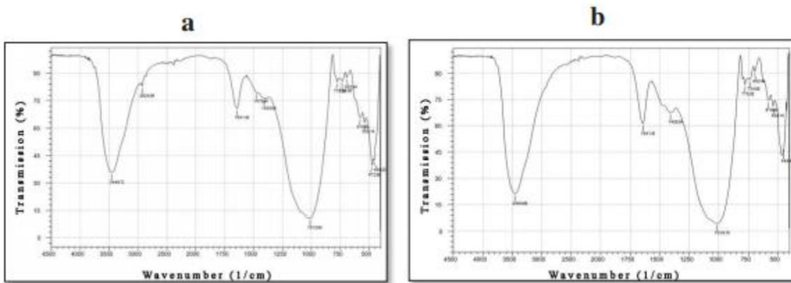
**FIGURE 5.** FTIR Spectra of (a) ACS based Geopolymer (b) GBFS based Geopolymer
