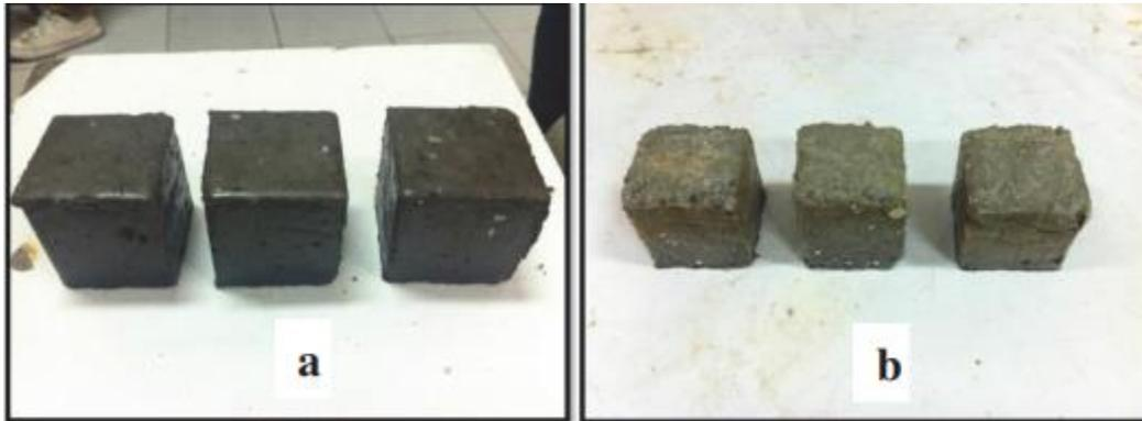
**FIGURE 2.** Geopolymer samples, prepared from fly ash, alkali activator, and (a) ACS or (b) GBFS
