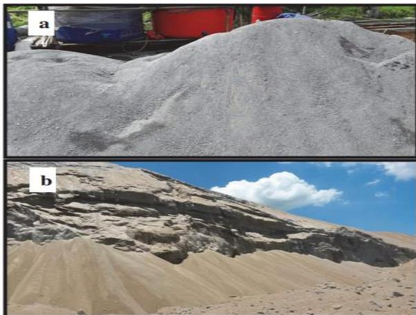
**FIGURE 1.** Air-Cooled Slag (a) and Granulated Blast Furnace Slag (b) in PT Krakatau POSCO
