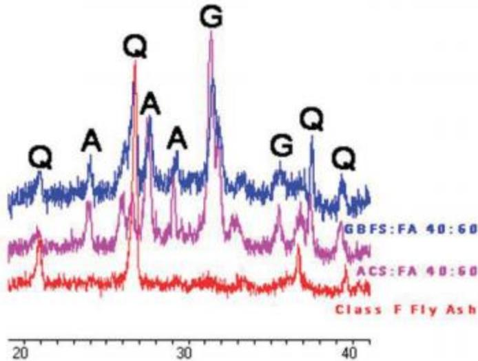
**FIGURE 4.** XRD diffractograms of class-F fly ash and Geopolymer. XRD peaks represent: A= Anorthite, G= Gehlenite, Q= Quartz. ACS:FA denotes ratio of air-cooled slag and fly ash in the samples, while GBFS:FA denotes ratio of granulated blast furnace slag and fly ash in the samples
