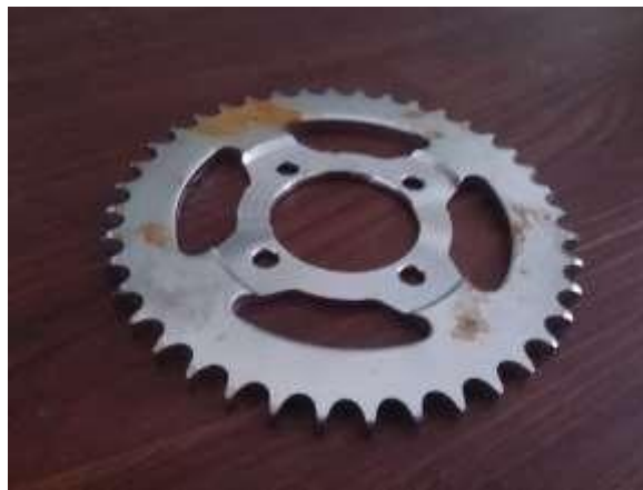
Gambar 6. Sprocket hasil powder metallurgy
